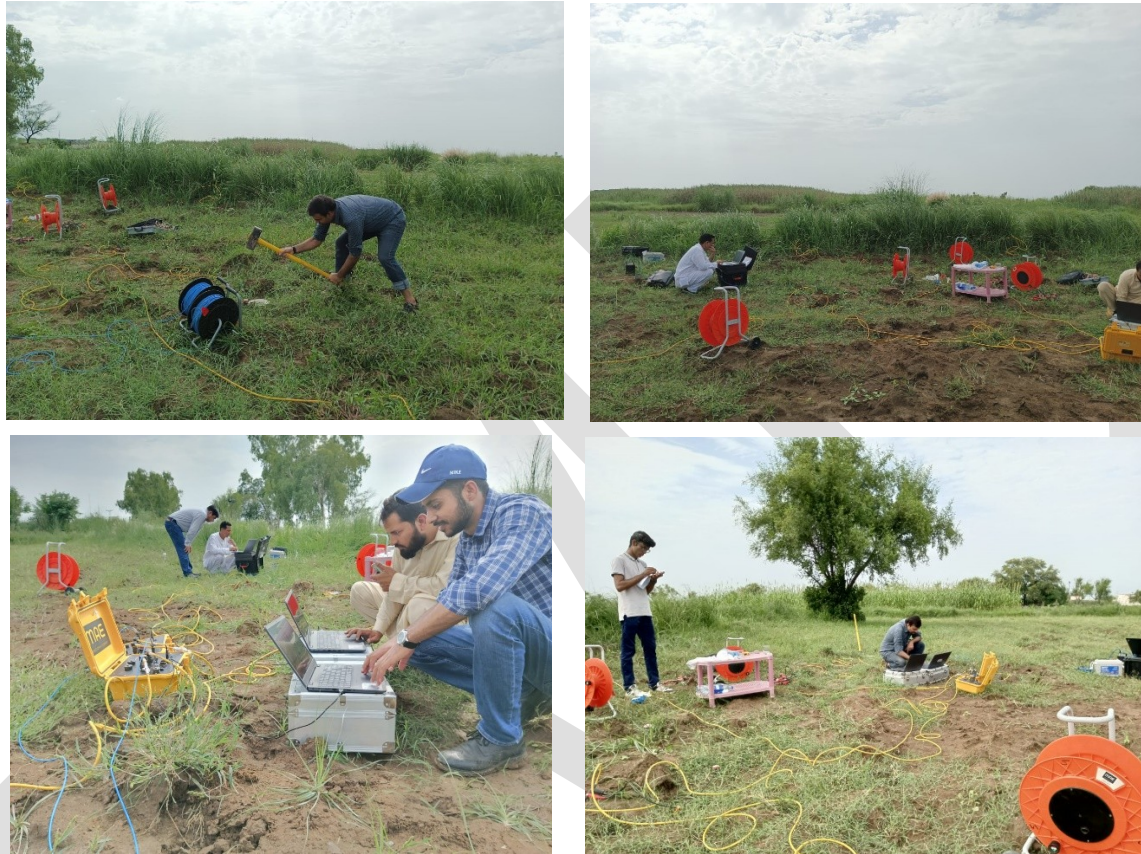
Figure 6. Field photographs from the geophysical survey near POL Well No. 10 showing MAM and MASW deployment for surface-wave site classification.
