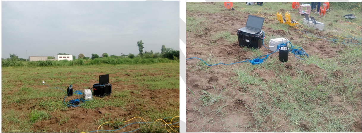
Figure 3. Field deployment of a short-period seismometer near Bahiya (POL area) for ambient-noise recording at stations BAH1 (left) and BAH2, (right) showing the three-component sensor, digitizer, power unit, and acquisition laptop used for HVSR and noise spectral analysis.
